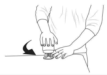
3 Push the side buttons on the main body to detach and remove.
